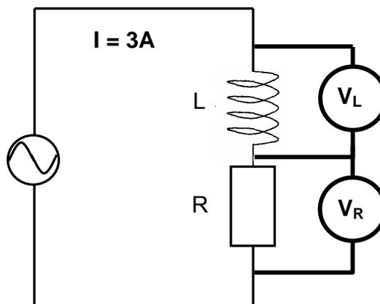
**FIGURE 5.1: R AND L CIRCUIT**
