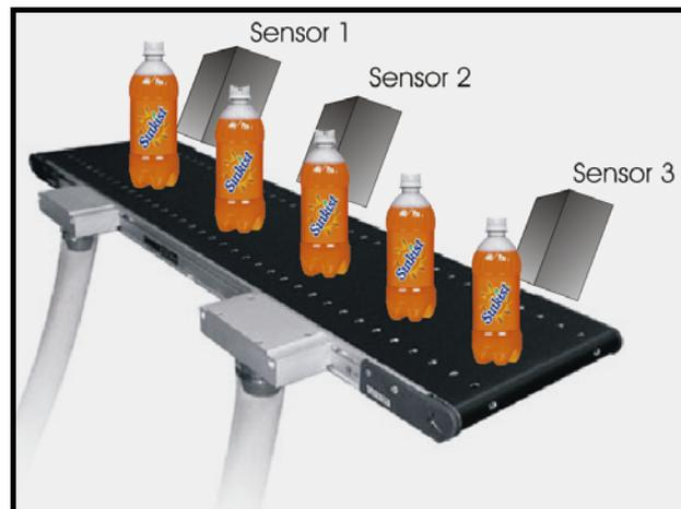
**FIGURE 9.2: CONVEYOR-BELT SYSTEM**
