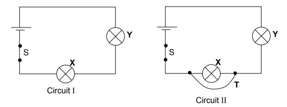
A wire T, of negligible resistance, is now connected across X as shown in Circuit II.
