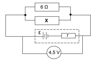
9.2.3 Calculate the resistance of **X** when the voltmeter reads 4,5 V. (5)
