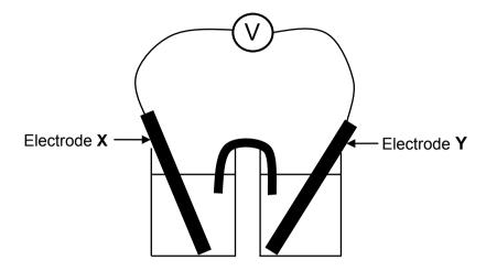
When the cell is functioning, ELECTRODE **X** GAINS MASS.
