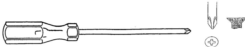
These screwdrivers have tips that are shaped to fit the crossed slots of Phillips head screws. For safe handling always select the correct size screwdriver with a properly shaped tip. Do not use the screwdriver as a chisel. Ensure that the tip of the screwdriver is inserted properly into the screw slot when using the screwdriver. Do not attempt to use a screwdriver that has no handle or a cracked or broken handle.
