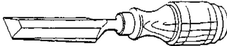
A bevel edge firmer chisel is used for paring and lighter work such as cleaning up corners of joints. Because of its bevel edge blade it is safe to pare through grooves without damaging the edges/ sides of the work piece.
