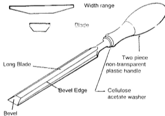
The paring chisel has a long thin bevelled edge blade and because of its light construction, is not for use with a mallet. For paring work such as finishing off joints and light shaping
