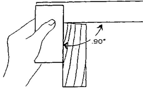
Testing for a right angle on a work piece
