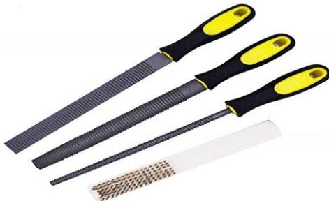
**Use:** A rasp is used to remove parts of timber quickly. It is used to shape concave and convex surfaces. Wood rasps have coarse teeth that are raised on the blade of the rasp. They have a very rough cutting action and tend to splinter the timber. Do not use a rasp without a handle or with a cracked or broken handle. Keep fingers away from the timber surface when the rasp is being used. Flat side for quick levelling and rounding of wooden materials.
