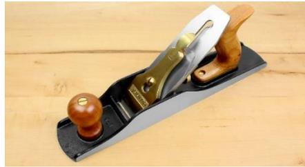
The jack plane is used to smoothen timber surfaces. As its name suggest it is a 'jack of all trades'. It is slightly bigger than the smoothing plane and will achieve perfect straight edges. Always keep the blade of the plane sharp and never drop the plane as the body is brittle. Store the plane on its side or with its blade above the sole of the plane so that the cutting iron will be protected.
