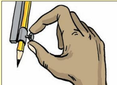
Set the compass to the radius of the circle. (The radius is the distance between the centre and the circumference; it is half the diameter.)
