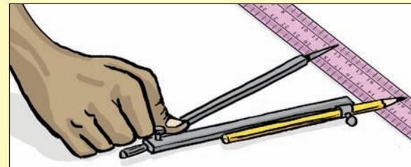
Make sure that the hinge at the top of the compass is tightened so that it does not slip.
