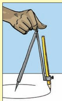
Align the pencil lead with the compass point.
