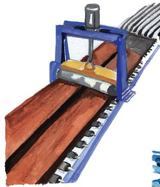
A machine is cutting up the clay mixture into strips.
