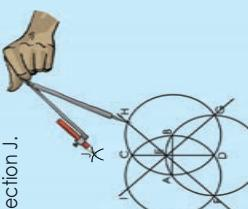
**Step 6:** Set your pair of compasses to the length of AI. Place the compass point on I, and make a small arc above C. Then place your compass point on H and make an arc crossing the first one. Label the point of intersection J.
