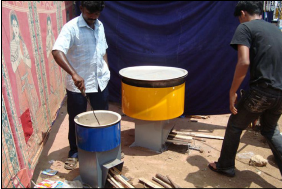
FIGURE A: ODOM stove prototype by the MOBY Institutional and Prakti Design Lab for burning smokeless, energy-efficient charcoal briquettes, using 70% less wood than traditional stoves (India), 2010.
