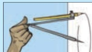
Set the compass to the radius of the circle. The radius is the distance between the centre and the circumference; it is half the diameter.
