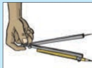
Press down the compass point and turn the knob at the top of the compass to draw a circle.
