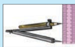
Make sure that the hinge at the top of the compass is tightened so that it does not slip.
