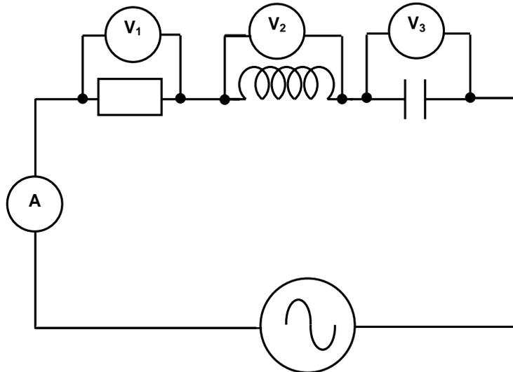
**FIGURE 5.1 – RLC SERIES CIRCUIT**
