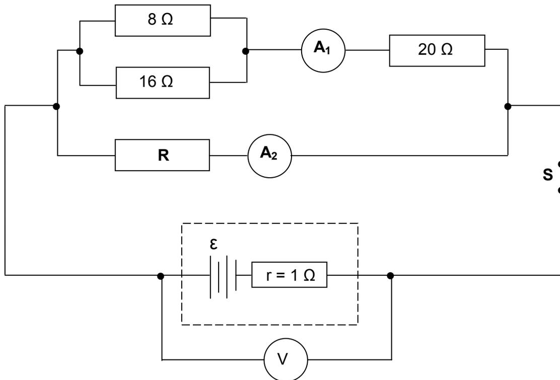
With switch **S** closed, the current passing through the  $8 \Omega$  resistor is  $0,5 \text{ A}$ .
