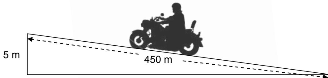
The total frictional force acting on the motorbike is 294 N. The combined mass of rider and motorbike is 300 kg. The average driving force on the motorbike as it moves up the incline is 350 N. Consider the motorbike and rider as a single system.
