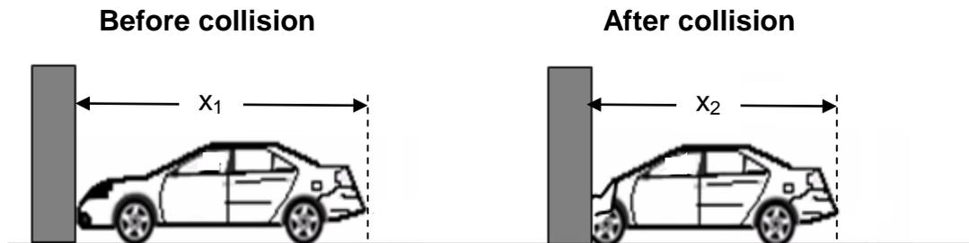
In one of the tests, a car of mass 1 200 kg strikes the barrier at a speed of  $20 \text{ m}\cdot\text{s}^{-1}$ . The crumple distance,  $(x_1 - x_2)$ , is measured as 1,02 m. (Ignore the effects of frictional forces during crumpling.)
