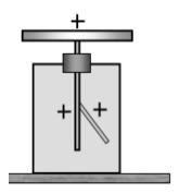
When an object is brought close to the plate, the leaves diverge more. We can therefore conclude that the object ...
