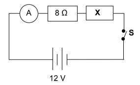
The 12 V battery has negligible internal resistance. When switch **S** is closed, the reading on the ammeter is 0,5 A.
