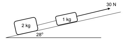
The kinetic frictional force between the 1 kg block and the inclined plane is 4 N while the kinetic frictional force between the 2 kg block and the inclined plane is 8 N.
