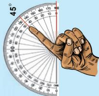
**Step 3:** Using (in this case) the inner scale, find the angle desired - here it is 45°.
