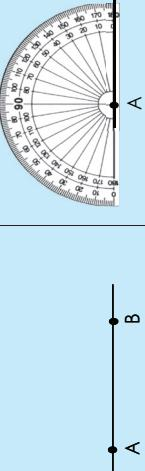
**Step 2:** Place the protractor so that the origin (small hole) is over point A. Rotate the protractor so that the base line is exactly along the line AB.
