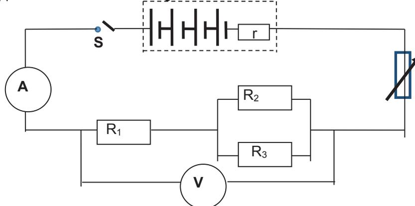
2. Close the switch and change the resistance in the rheostat and take the ammeter and voltmeter (terminal voltage) readings and record in Table 2. (Open the switch while recording the readings in order to spare the batteries' life span). Repeat step 10 two more times.
