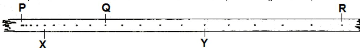
12. Count 5 dots of the first displacement **PQ** and mark with an **X**, count 5 dots for the second displacement **QR** and mark with a **Y**. See figure above.
