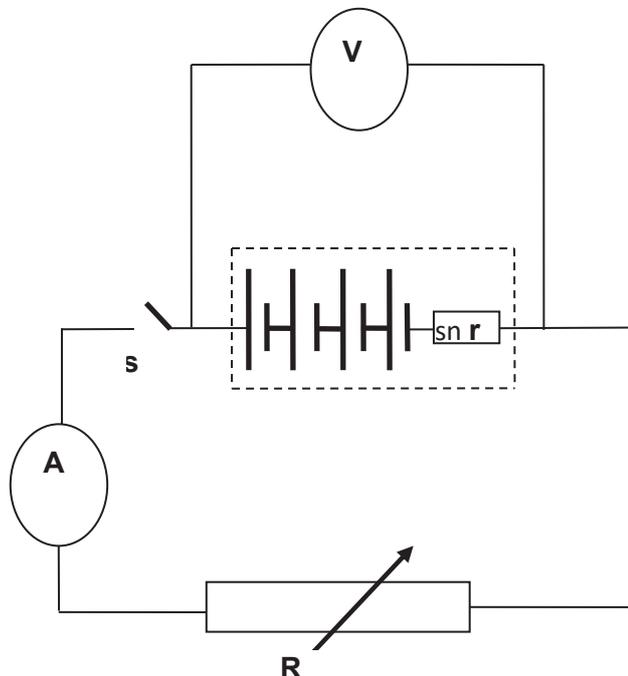
2. Note the voltmeter reading when the switch **S** is open and record in the *Table 1* below.
