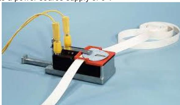
4. Select in the ticker-timer the frequency (number of dots in one second) of 40 Hz or 50 Hz.
