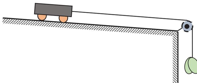
9. Place the unused masses provided on the trolley. You are going to transfer them to the mass holder each time the accelerating force is increased. This ensures that the total mass experiencing acceleration remains constant throughout the experiment.
