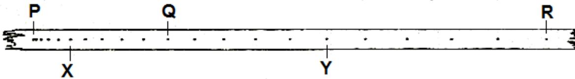
11. Count 5 dots of the first displacement **PQ** and mark with an **X**, count 5 dots for the second displacement **QR** and mark with a **Y**. See figure above.
