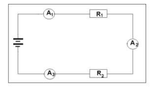
How does the reading of A<sub>2</sub> compare to the reading of A<sub>1</sub> and A<sub>3</sub>?
