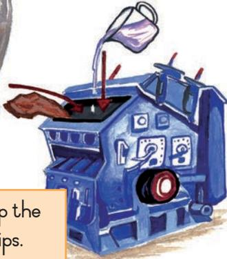
Clay is ground up finely and mixed with water.
