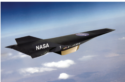
Figure 12.18 NASA's scramjet, the X-43 flies at 7 000 km/h.
