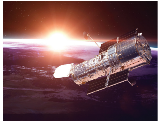
Figure 13.23 The Hubble Space Telescope has a 2.4m diameter collecting mirror.
