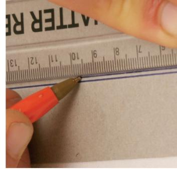
Figure 19: Make a fold by first making two grooves on the inside.
