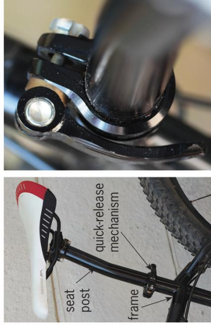
Figure 12: A quick-release mechanism is used to clamp the seat post to the frame of this bicycle.
