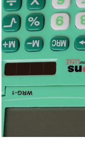
Figure 15: Photovoltaic cells in a calculator
