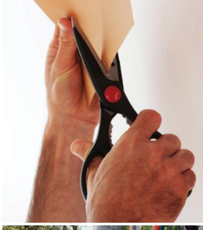
Figure 16: A pair of scissors is a pair of linked first-class levers.
