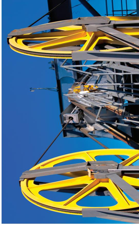
Figure 2: This photograph shows detail of sheave wheels used for pulling in a cable. The sheave wheels in the photograph are used for a cable car, but they are similar to the sheave wheels used on a mine's winch system.
