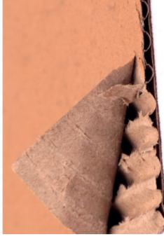
Figure 11: Large boxes are made of corrugated cardboard.
