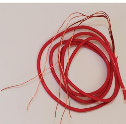
Copper wire, 1 mm (this bends easily by hand and can be cut with scissors; buy from hardware store)
