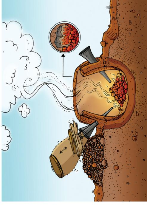
Figure 12: Illustration of how an early iron smelter was constructed and used
