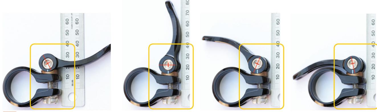
Figure 13: The sides of the quick-release mechanism move or clamp closer together as the eccentric cam is turned by the handle.
