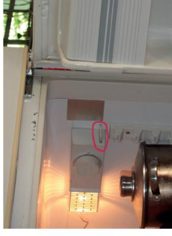
Figure 5: Find the switch for the fridge’s light.
