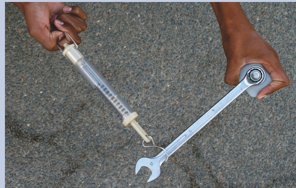
Figure 4.21 The spring balance is attached to the ring of the spanner, with the other end of the spanner on a nut.
