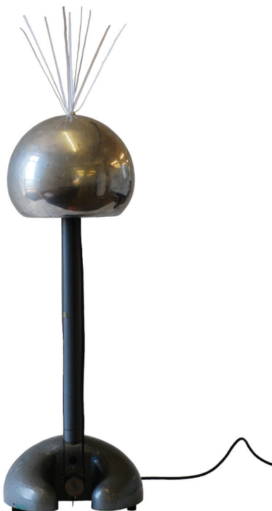
Figure 12.20 The paper strips repel each other away from the dome.
