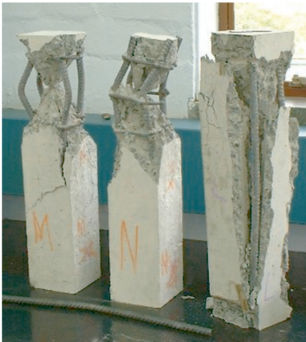
Figure 3.21 Compression failure in a concrete column. The concrete has broken away and the reinforcing bars have buckled.
