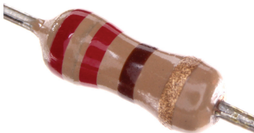
Figure 14.4a The colour bands are red, red, and brown, with a gold band at the end.
