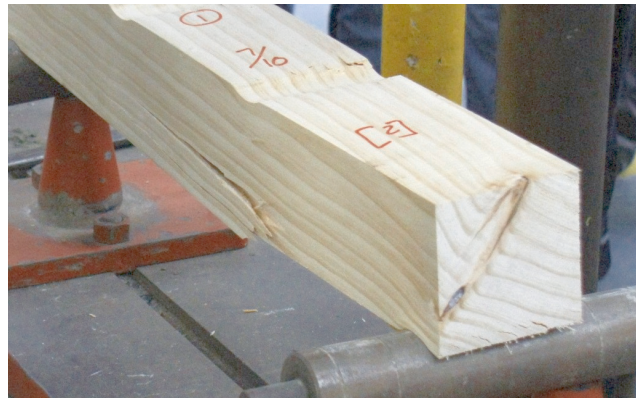
Figure 5.25 Shear in this piece of wood probably started when the fibres at the bottom of the beam failed in tension.
