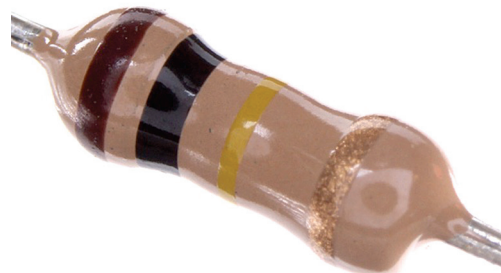
Figure 14.4b The colour bands are brown, black, and yellow, with a gold band at the end
