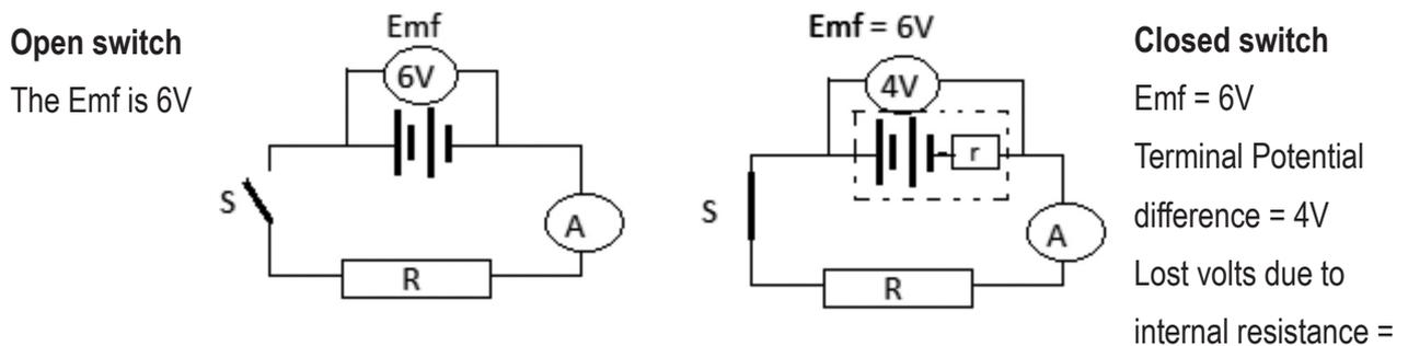
What happens to the lost volts when the external resistance is increased?
