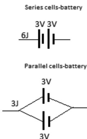
The cell/ battery is the source of energy. It transfers energy to every coulomb of charge that passes through it. When a cell is marked 3V, it means that it can **transfer 3J of energy** to every coulomb of charge passing through it.
