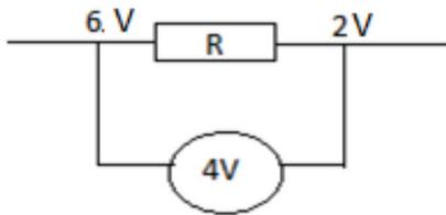
It measures the potential difference (energy delivered) across the resistor. Therefore it is connected in parallel across the resistor. It measures the voltage before and after the charges pass through the resistor and then calculates the difference, i.e.
