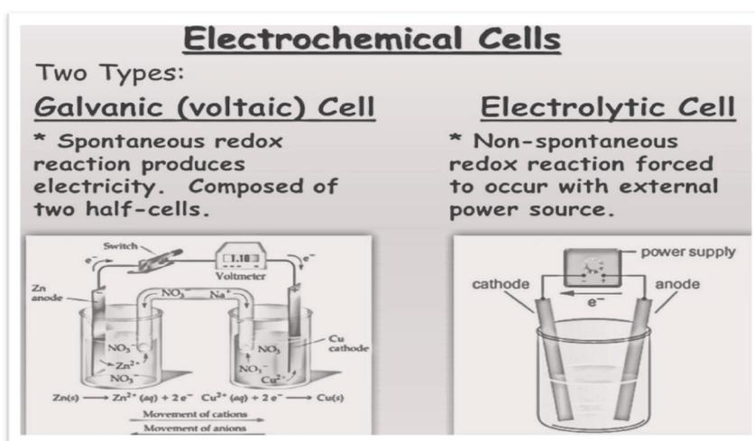
While the galvanic cell **produces** electricity, the electrolytic cell **needs** electricity.
