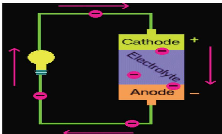
An **electrode** is a **conductor** that is used to make contact with a non-metallic part of a circuit. This could be a gas or an aqueous solution.
