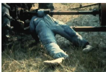
Simulation of PTO danger. An overall sleeve caught by an open PTO.
