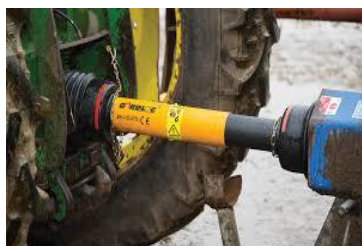
Protected PTO shaft of a tractor to prevent injury.
