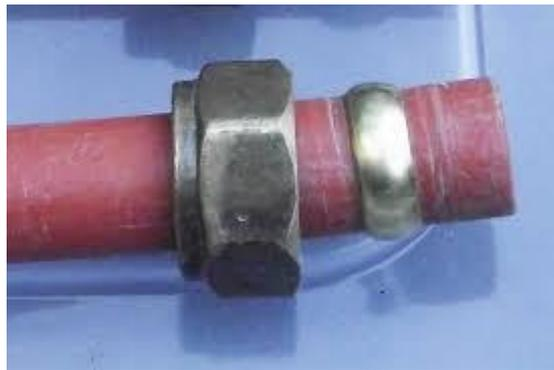
Brass Compression joint with lock ring and nut.
