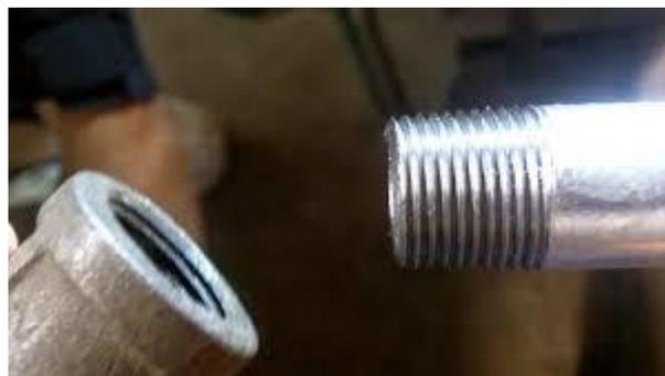
Pipe with screw thread can now be connected to any galvanized fitting.
