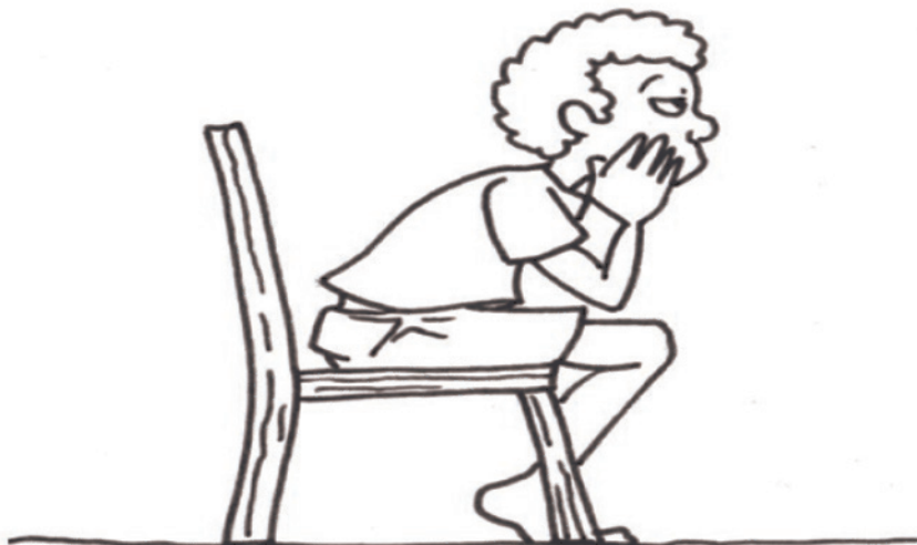
Figure 1. A boy sitting on a chair is exerting a pushing or compression force on the chair. As long as a person sits still on the chair, the force on the chair remains in the same place. This is called a stationary or static force.
