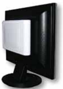
Figure 6: Thin client computer mounted on back of LCD monitor
